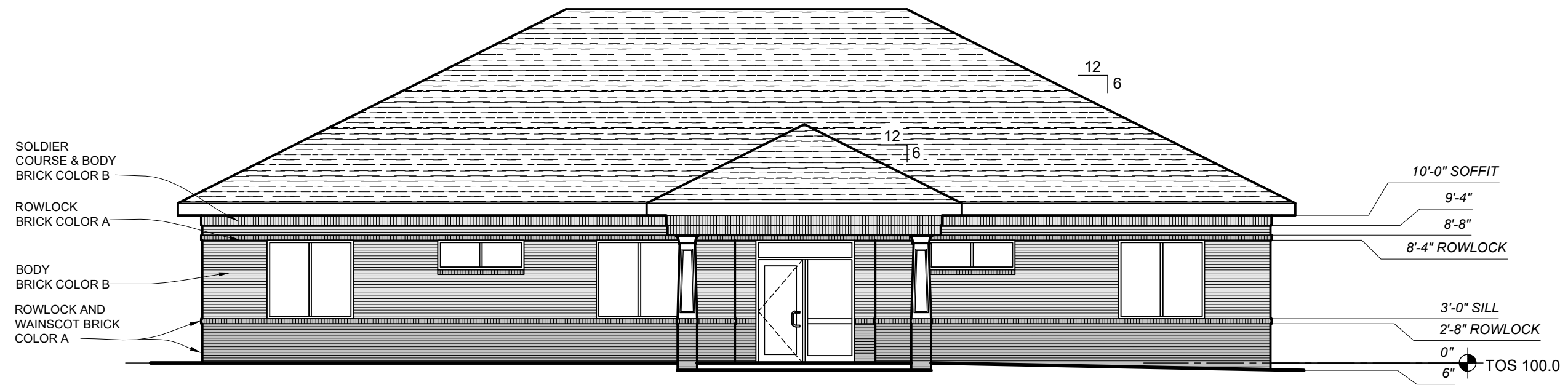
FRONT EXTERIOR ELEVATION
